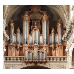
When the keyboard is struck, it opens the pipe hole to let air be blown through making sound. The bigger the pipe, the lower the pitch of the sound.
